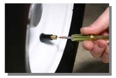
Position the valve stem between the 4 and 8 O'clock position and remove the valve stem. The tire will deflate. (fig. 1)
