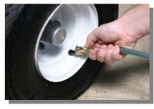
Attach the brass connector from Arnco's ReSeal pump to the valve stem (fig. 2)
