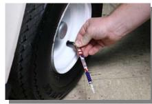
Inflate tire and check for proper operating pressure. (fig. 4)
