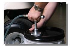
Pull up on the handle and inject the proper mount of ReSeal into the tire. Each stroke delivers 6 ounces. (fig. 3)
